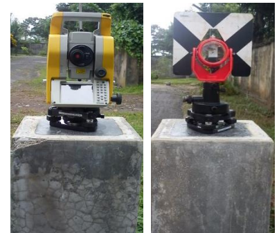
Figure 03: Instrument & Tribrach on the Pillar
